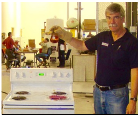
John Lentini in controlled experiment to determine the flammability of Captain Morgan's Spiced Rum.
