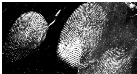
Latent fingermarks identified on aluminium foil using the immunogenic method developed by Dr. Xanthe Spindler (Dr. Xanthe Spindler)
